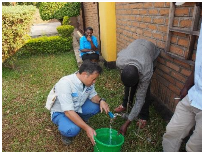
Meter accuracy test in the field
