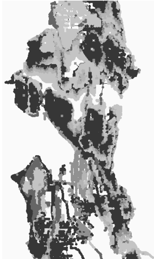
Figure 3. Estimated SPU System Water Pressure Three Hours After Major Earthquake (Darkest Areas Denote Water Pressure = 0)
