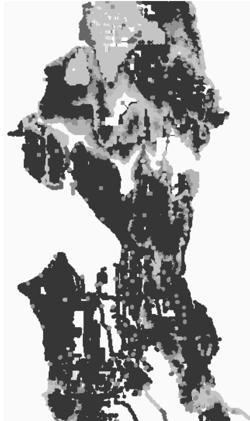
Figure 4. Estimated SPU System Water Pressure Ten Hours After Major Earthquake (Darkest Areas Denote Water Pressure = 0)
