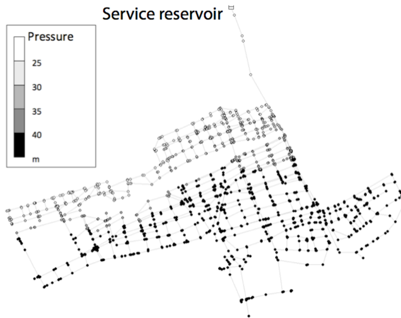
Figure 3. Map of water pressure in Nada network in normal condition
