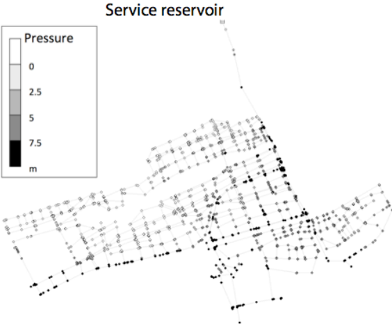
Figure 5. Map of water pressure in Nada distribution network after the earthquake disaster
