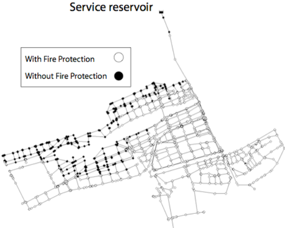
Figure 6. Map of nodes with fire protection function in Nada distribution network after the event
