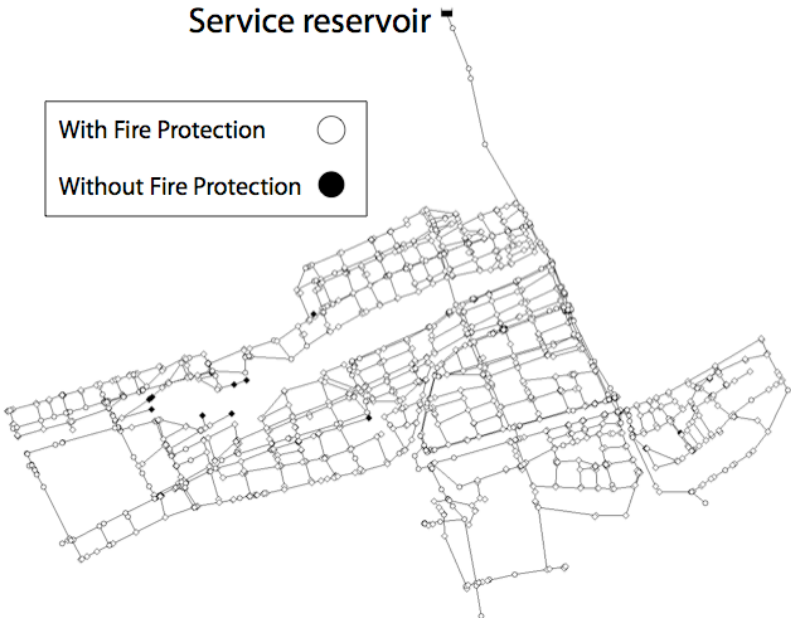
Figure 4. Map of nodes with fire protection function in Nada distribution network
